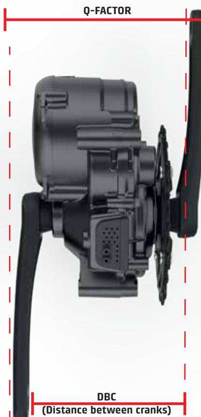
When choosing the components of your E-Bike, be sure to check the Q-Factor and the DBC to prevent the cranks from touching the frame, and to verify that there is no misalignment of the cranks with the center of the bike.
