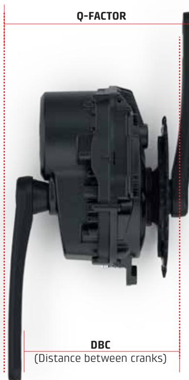
When choosing the components of your E-Bike, be sure to check the Q-Factor and the DBC to prevent the cranks from touching the frame, and to verify that there is no misalignment of the cranks with the center of the bike.
