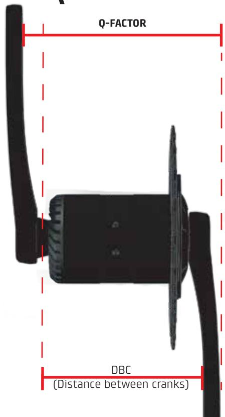
When choosing the components of your E-Bike, be sure to check the Q-Factor and the DBC to prevent the cranks from touching the frame, and to verify that there is no misalignment of the cranks with the center of the bike.
