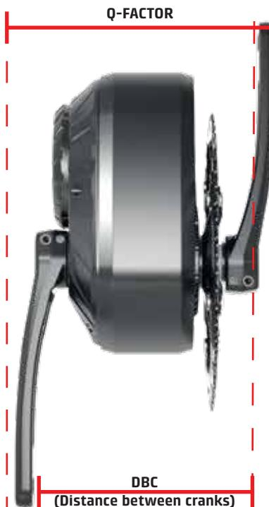
When choosing the components of your E-Bike, be sure to check the Q-Factor and the DBC to prevent the cranks from touching the frame, and to verify that there is no misalignment of the cranks with the center of the bike.
