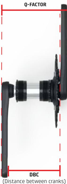
When choosing the components of your E-Bike, be sure to check the Q-Factor and the DBC to prevent the cranks from touching the frame, and to verify that there is no misalignment of the cranks with the center of the bike.
