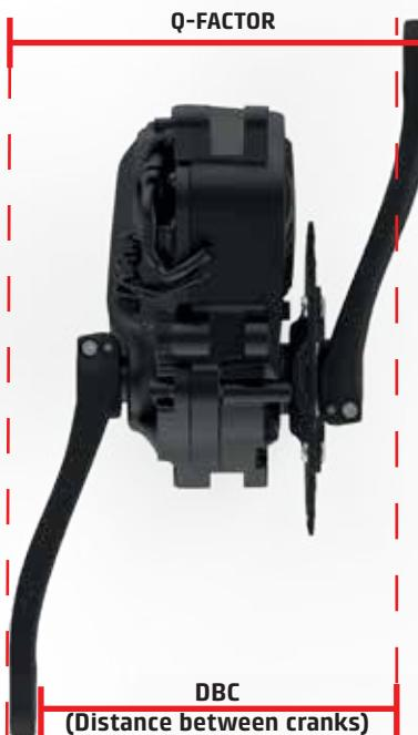
When choosing the components of your E-Bike, be sure to check the Q-Factor and the DBC to prevent the cranks from touching the frame, and to verify that there is no misalignment of the cranks with the center of the bike.
